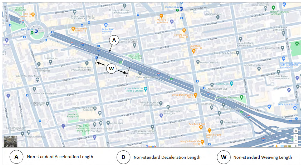
Figure 7.15. Cross Bronx Between White Plains Rd and Zerega Ave. Non-Standard Ramps & Weaving Sections. Source: Google Maps
