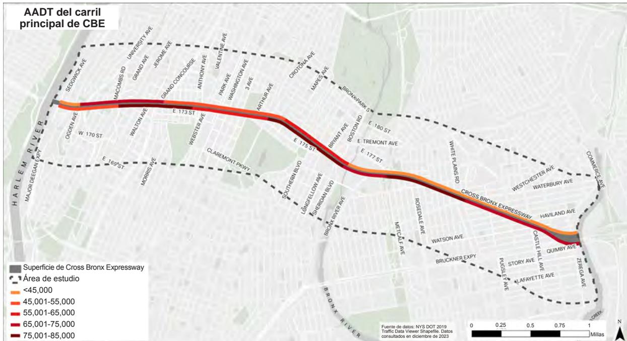
Figura 2.3. AADT direccional del carril principal de Cross Bronx. Fuente: NYSDOT Traffic Data Viewer 2019
